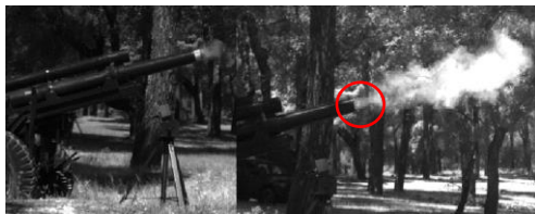
Figure 14: Liberation of gases before and after the projectile
