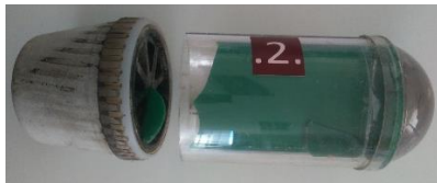
Figure 21: Projectile that broke inside the barrel
